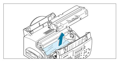
3. Remove the jammed paper by carefully pulling it out of the machine.
